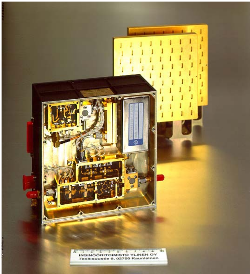
Fig.5. The Radar Electronics and (behind) the Antenna.
