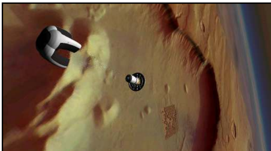
MTSV cross parachute. A cross parachute, impregnated with an ablative material, was added when it was realized there may be high temperatures (and high mechanical loads).
